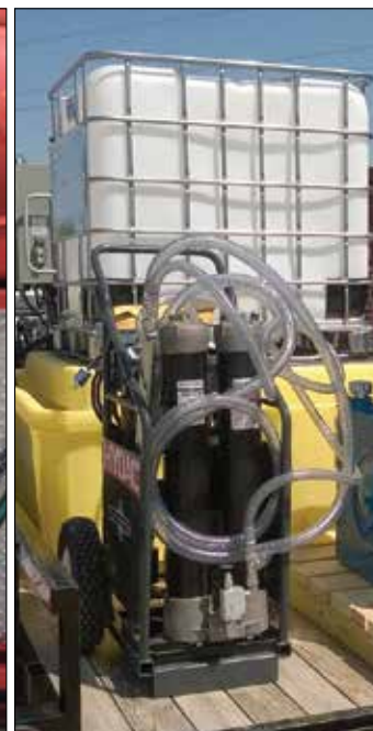
OFS Filtration Station with HPU.
